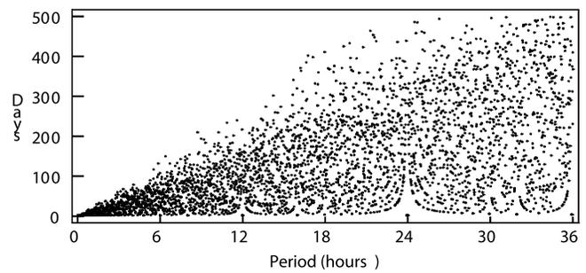
FIG. 2.—Number of days until a second opportunity for detection using the Ohio State transit telescope, for sources with periods up to 36 hr. Prospects are especially poor for sources with periods near but not equal to the terrestrial 23.9345 hr day.
