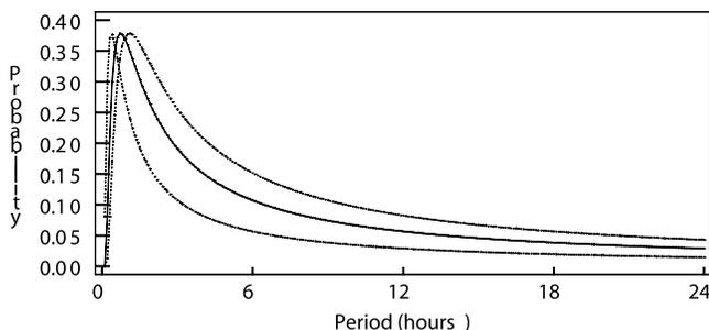
FIG. 1.—Probability of exactly one detection in 18 trials. The solid line represents a signal duration of 144 s every  $n$  hours. The upper dotted line represents a signal duration twice as long, the lower dotted line half as long. The probability of exactly one detection falls off rapidly for periods less than about 1 hr as a result of multiple detections.
